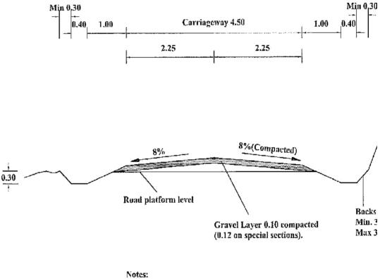
1.All dimensions in metres 2.Gravel thickness may be increased as directed by the Engineer
