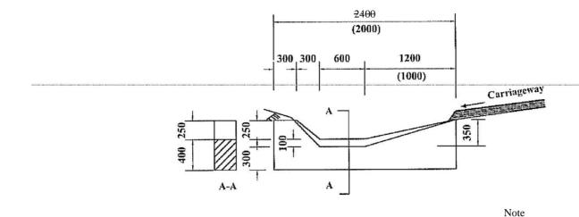
SECTION OF MASONRY SCOUR CHECK
