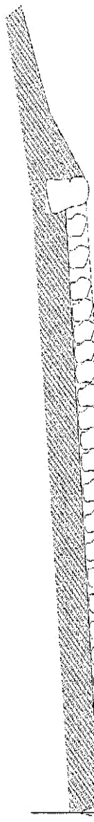
3. EDGE BEAM SECURED AND LARGE STONES LAID ON EDGE
