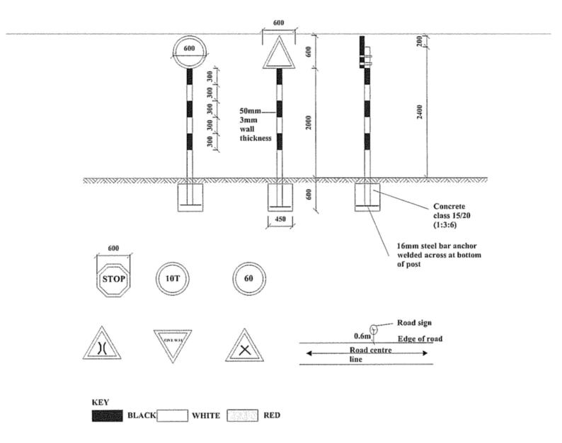
1. The type of sign required and their location shall be as shown on the Road Plan or as directed by the Engineer. 2.Sign plate to be 2mm thick mild steel plate
