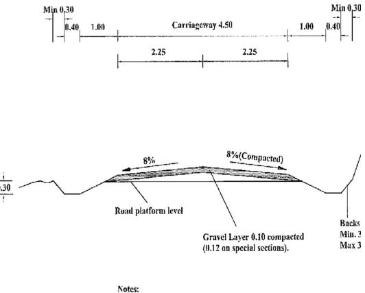
1.All dimensions in metres 2.Gravel thickness may be increased as directed by the Engineer
