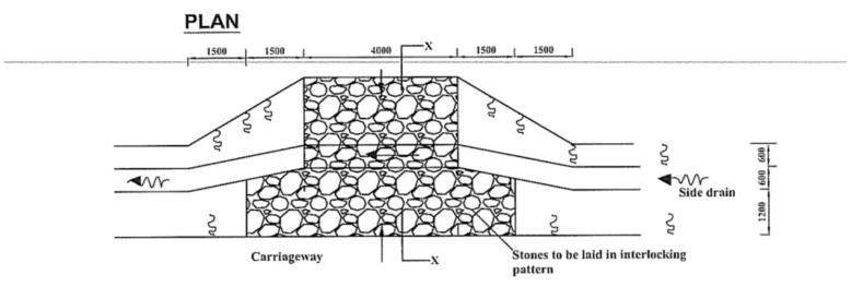
150mm Grouted Stone Pitching (Cement mortar 1:4)
