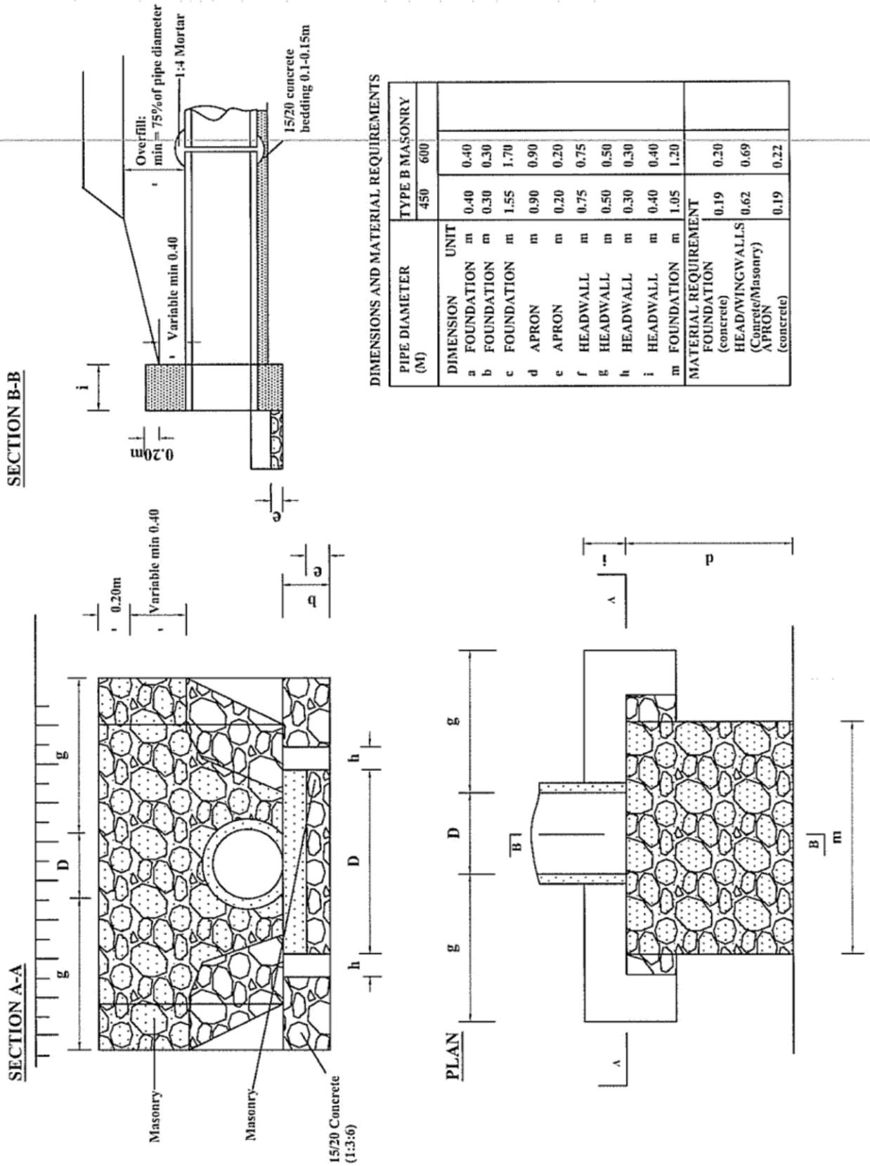
FIGURE C15-HEADWALL TYPE 4( FOR ACCESS CULVERTS)
