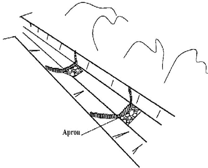
Scour checks made of stones
