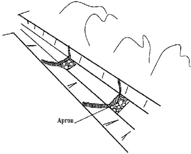
Scour checks made of stones
