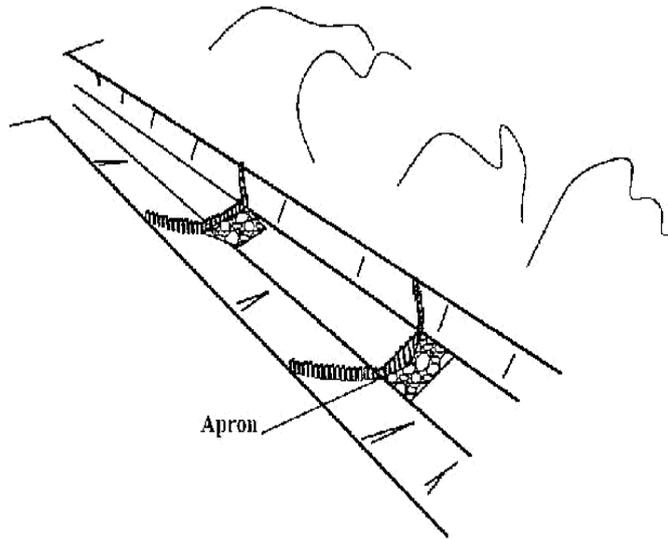
Scour checks made of stones
